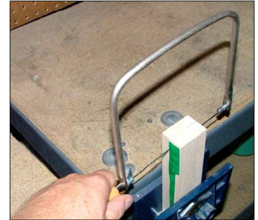
Figure 13: Securely clamp block in vise. Then carefully cut the block. After you cut half way through, turn the block over and finish cutting from the other side.
