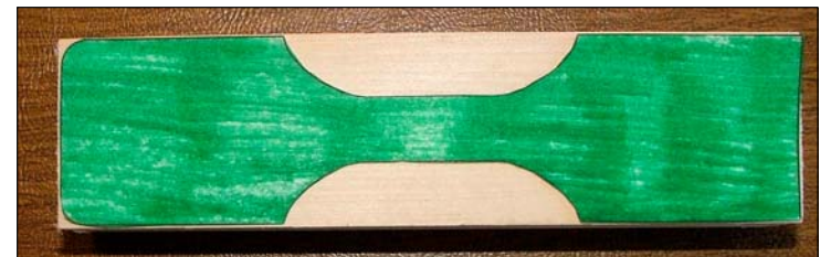
Figure 14: Top template attached to block
