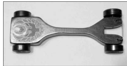
Figure 85: Aerodynamic, very little wood in center or front of car
