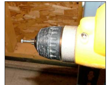
Figure 32: Insert axle in drill leaving half an inch exposed.
