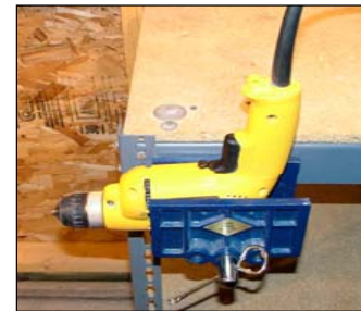
Figure 31: Clamp drill in vise. Be sure not to clamp too tight.
