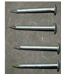
Figure 97: This set of axles is straight.
