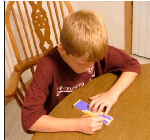
Figure 5: Tracing car design on to pine block. In this photo Tanner is using a pattern cut from blue paper. He then traces the pattern onto his pine block using a pencil.
