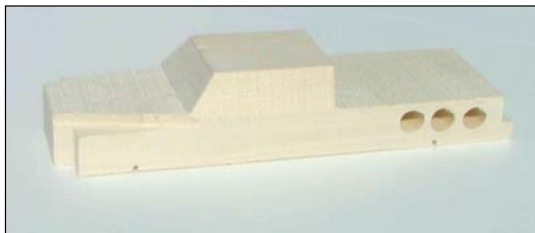
Figure 113: Weight holes drilled in rear of truck design.
