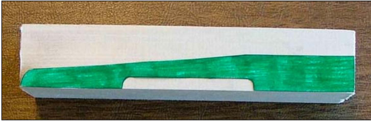
Figure 10: Side view template attached to block
