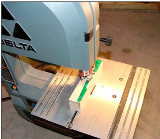
Figure 11: Cutting the block using a ban saw
