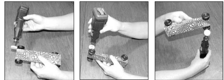
Figures 81, 82, and 83: Spin the wheels in all three positions.
