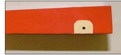
Figure 52: Tape removed after painting
