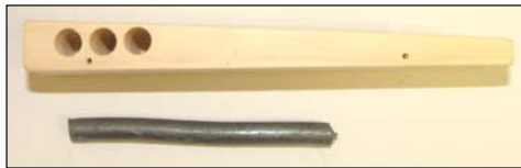
Figure 25: Holes drilled in side of car. Lead wire or fishing weights fit into each hole. The holes are then covered with wood putty before painting.
