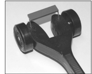
Figure 92: If you are racing with an electronic timing system, then you may want to use a quick start bar like the one shown in this photo. The wider bar will help the electronic sensors detect the front of the car as it crosses the finish line.
