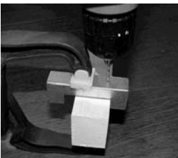
Figure 4: Drill Raised Axle Hole
