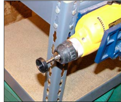
Figure 37: Attach wheel to drill using mandrel
