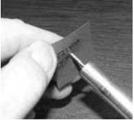
Figure 9: Apply Course-Grit Sand Paper
