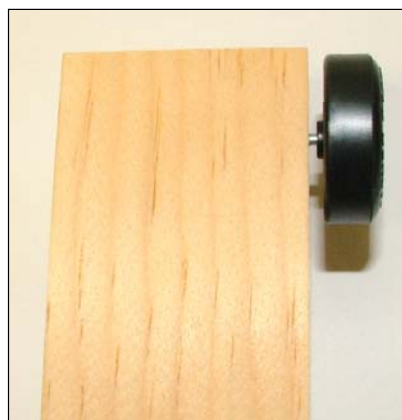
Figure 21: Wheel properly spaced from car body when using drilled axle holes. Drilled axle holes are discussed on page 45.
