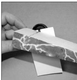
Figure 19: Using wheel spacer to attach wheel
