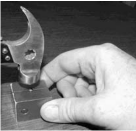
Figure 14: Lay press on its back and strike axle head.
