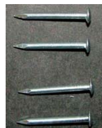
Figure 96: This set of axles is NOT straight.
