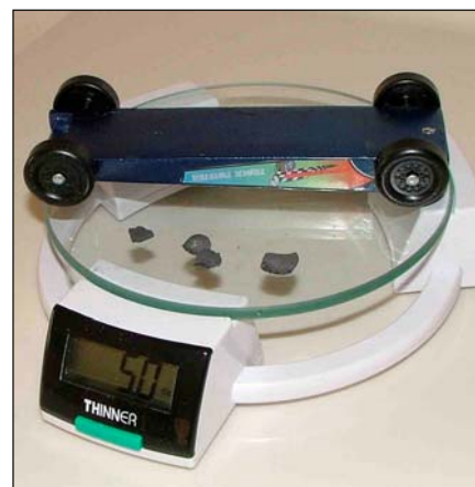
Figure 84: Car placed on scale upside down with small bits of lead putty added for maximum weight.
