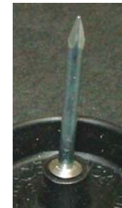
Figure 34: Photo of axle with burrs removed.
